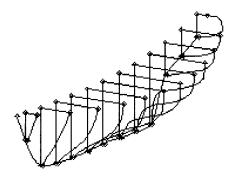
Figure 4.5. Solid-based surfacing technique
