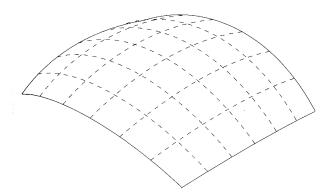
Figure 4.3. A surface modeled shell
