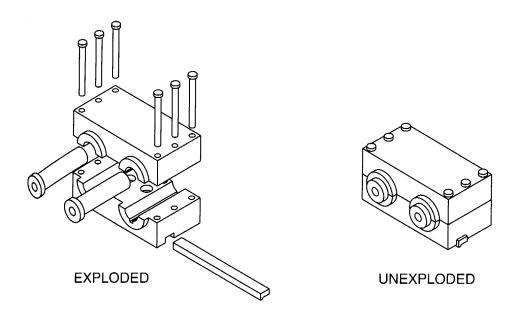
Figure 12.4. Exploded and unexploded assemblies
