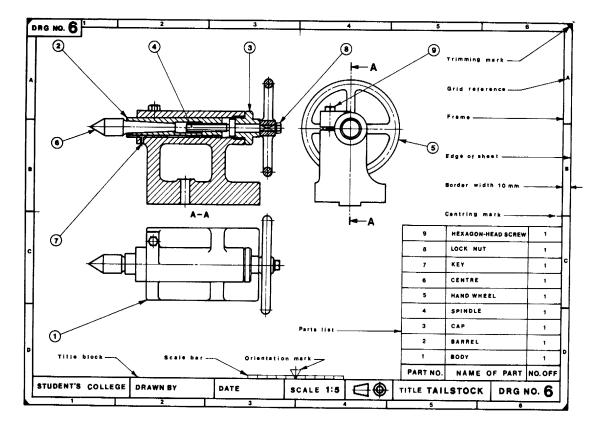
Figure 12.3. Assembly drawing with explanatory notes
