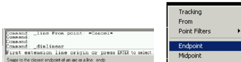
Then you may give the second and the last point to measure the dimension. Again Endpoint osnap command will be used as shown below.
